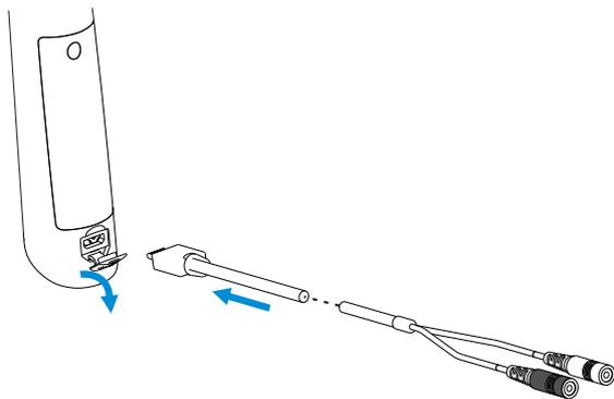
Insert lip hook into white slot, insert file clip into black slot.
