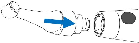
The contra angle can be 340 degrees rotated without take off, make it easy to watch the LCD in treatment by rotating the contra-angle.
