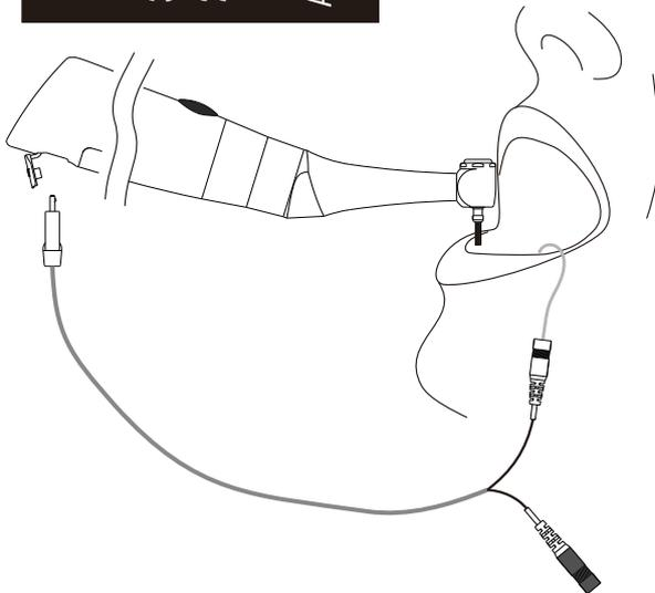
When using motor combine apex function, the measure wire must be connecting with motor by USB socket, and white slot connects with lip by lip hook, keep the black slot idle.
